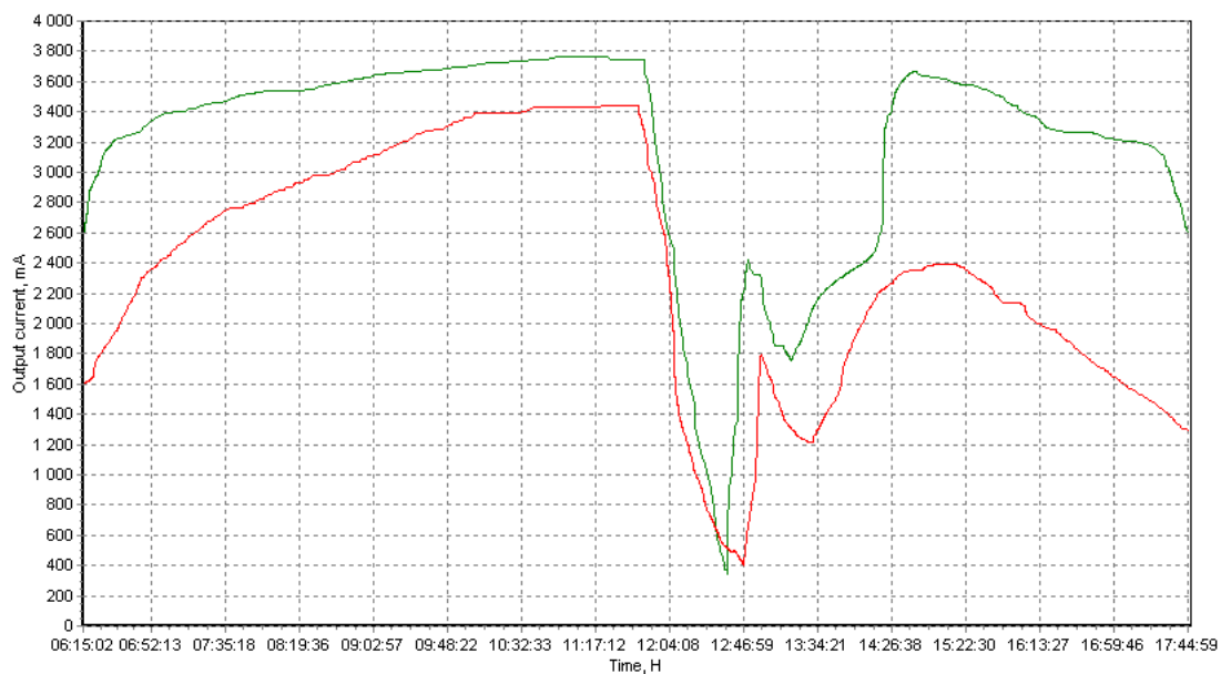
Fig.16: Temporal representation of voltage generated by dual-axis tracker and fixed panel
