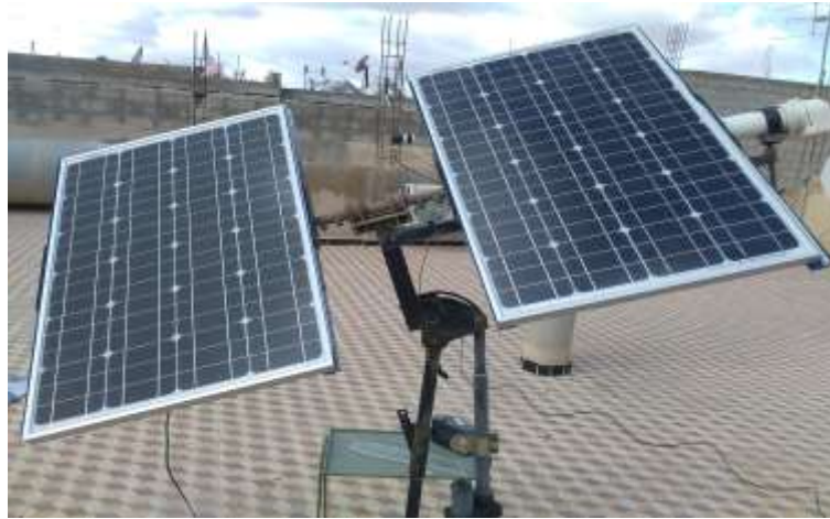
Fig.4: Structural design of our proposed dual-axis solar tracker
